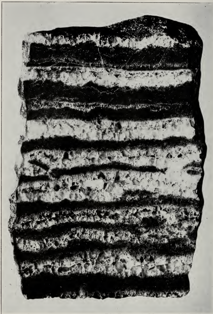
FIG. 35. Diffusion banding in fluoritic material from Lead Hill. The individual bands of coarse fluorite (white in the photograph) are \frac{1}{2} to \frac{3}{4} inch wide. (After Bain, H. Foster, Fluorspar deposits of southern Illinois: U. S. Geological Survey Bull. 255, Pl. V, 1905.)
